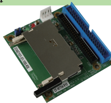
IDE to CF Type II converter board with master/slave mode selection
